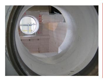
Vulcasil A99I is a +99% bubble alumina insulation material designed for use in reducing atmospheres such as hydrogen where the presence of silica is not permitted. Its resistance to hydrogen attack at high temperatures makes it ideal for use in bright annealing furnaces where Vulcan Refractories have unrivalled experience. Vulcasil HI 99 is also used as a backup lining in ammonia reformers and in areas where high purity insulation is required up to 1850°C.
